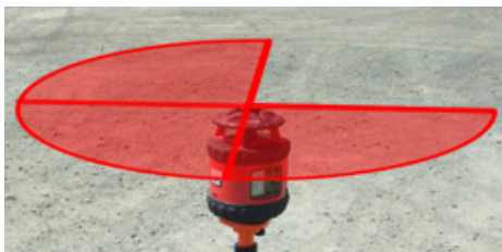
LCD and photo showing one quadrant turned off.
