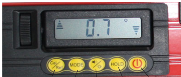
Self Calibration & Reference Units of Measure Sound & Light On/Off Hold Power On/Off
