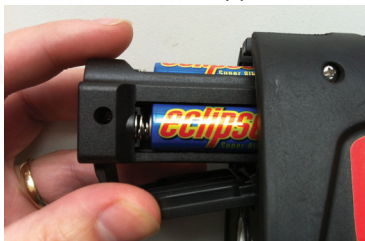
Note: Insert in direction of arrow on battery/holder.
