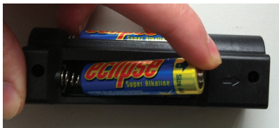
Installing "AA" Alkaline batteries into the battery holder.
