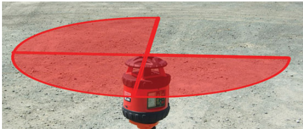
Photo showing one quadrant (90° arc) of rotation with laser output turned off
